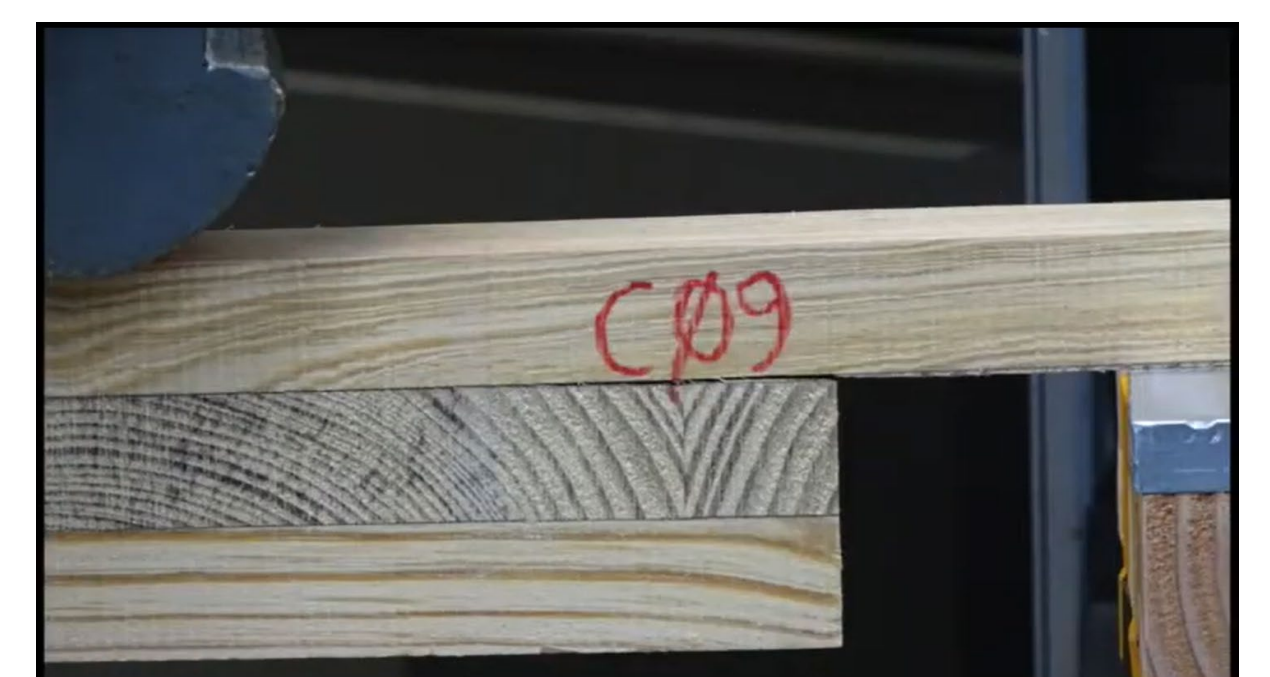
Notched CLT Delamination test @ depth 2 layers
